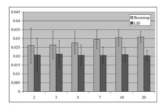
Figure 18. Tracking error for time step 10, as a function of the number of ships to be tracked for the bootstrap filter and LIS. Both algorithms use the same number of particles. The statistics is obtained by running 100 experiments for 10 independent realizations.
