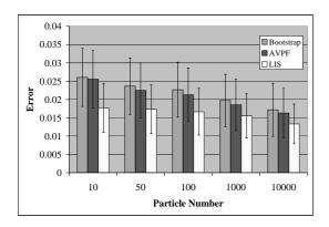
Figure 17. Tracking errors of the bootstrap filter, AVPF and LIS and the deviation of the error with different particle sizes when tracking 3 ships
