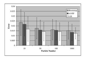
Figure 8. Tracking errors of the bootstrap filter, AVPF and LIS and the deviation of the error as a function of the number of particles
